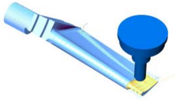
5-axes machining with material removal
